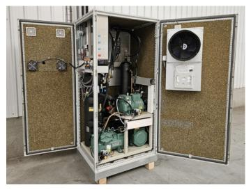
The supplied switch box is equipped with the control of the cell and two Danfoss drives.
